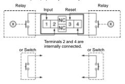
Note: Use Relays and Switches that have high contact reliability because the current flowing from terminals 1 or 3 is as small as approx. 10 μA. OMRON's G3TA-IA/ID is recommended as the SSR.
