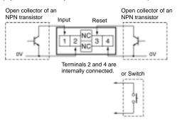
Note: 1. Residual voltage in the output section of Proximity Sensors or Photoelectric Sensors becomes less than 0.5 V because the current flowing from terminals 1 or 3 is as small as approx. 10 μA, allowing easy connection.
